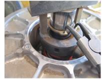
12) Be certain to properly align the "MASTER" spline for the spring retainer cap when re-installing.
